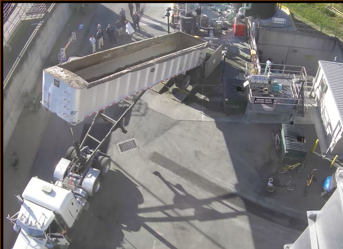
Tested food waste delivery from Republic Services, 20 tons, using widened floor hatch in May 2024
